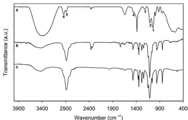
**Figure 5.** FT-IR spectra of silanized ferrofluids (a) (significant IR bands (1) 1040  $\text{cm}^{-1}$ ; (2) 1108  $\text{cm}^{-1}$ ; (3) 1199  $\text{cm}^{-1}$ ; (4) 1434  $\text{cm}^{-1}$ ; (5) 2868  $\text{cm}^{-1}$ ; (6) 2914  $\text{cm}^{-1}$ ), pure PEG (b) and PEGylated ferrofluids (c).
