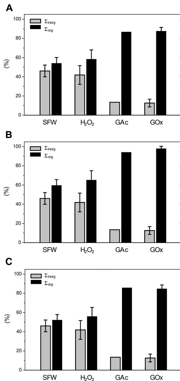
**Fig. 4.** Evolution of the molar concentration ratio of the sum of organic elements ( $\Sigma_{org} = C + O_{org} + N$ ) and the sum of inorganic elements ( $\Sigma_{inorg} = Cu + Ni + O_{inorg} + Cl$ ) measured by XPS (data from Table 3), on 90Cu-10Ni samples after immersion period of 5 days in SFW, H<sub>2</sub>O<sub>2</sub>, GAc and GOx.  $O_{org}$  was computed using (A) Eq. (3), (B) Eq. (4) and (C) Eq. (5). The standard variations are the mean value of 3 independent measurements.
