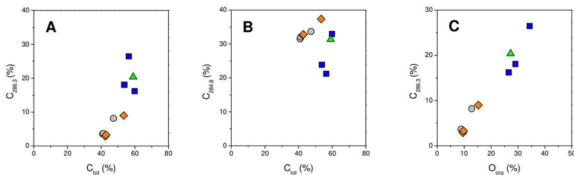
**Fig. 7.** Relationship between molar concentrations measured by XPS recorded on 90Cu-10Ni samples after immersion in SFW (●), H<sub>2</sub>O<sub>2</sub> (◆), GAc (▲) and GOx (■). O<sub>org</sub> was computed using Eq. 3: (A) C<sub>286.3</sub> vs C<sub>tot</sub>, (B) C<sub>284.8</sub> vs C<sub>tot</sub>, (A) C<sub>286.3</sub> vs O<sub>org</sub>.
