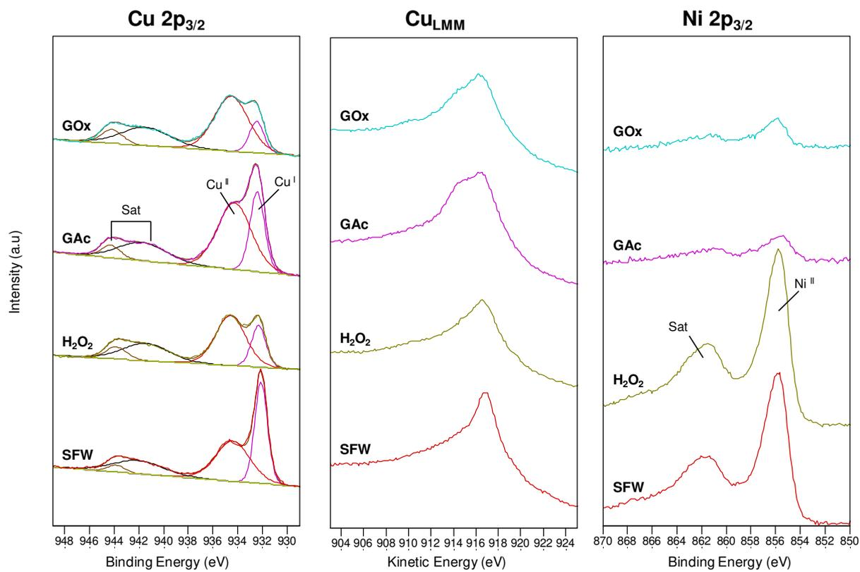
**Fig. 3.** Representative Cu 2p<sub>3/2</sub>, Cu L<sub>3</sub>M<sub>45</sub>M<sub>45</sub> and Ni 2p<sub>3/2</sub> peaks recorded on 90Cu-10Ni samples after immersion period of 5 days in the different media: SFW, H<sub>2</sub>O<sub>2</sub>, GAc and GOx.
