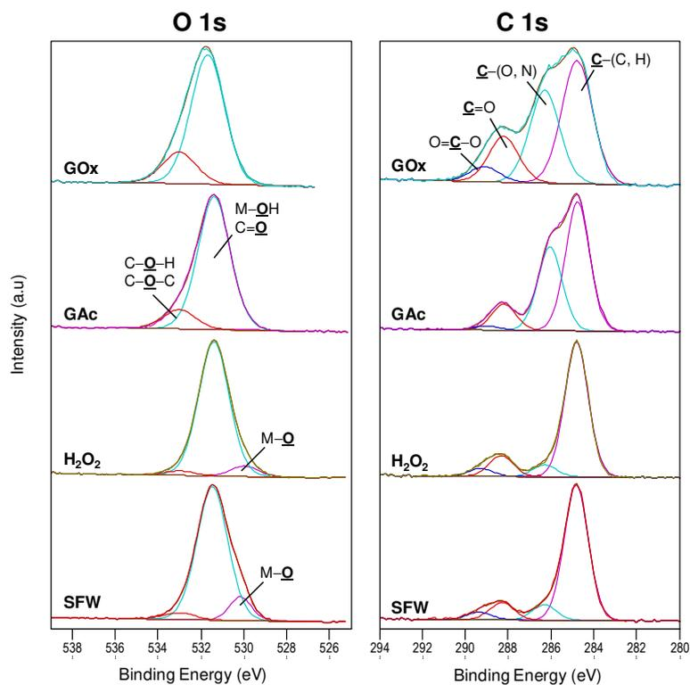
**Fig. 2.** Representative O1s and C1s peaks recorded on 90Cu-10Ni samples after immersion period of 5 days in the different media: SFW, H<sub>2</sub>O<sub>2</sub>, GAc and GOx.
