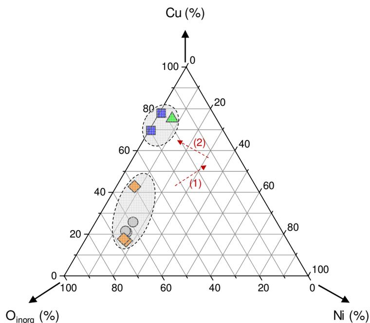
**Fig. 5.** Ternary diagrams presenting the sums of mole fractions determined by XPS: (A) elements related to the inorganic matter Cu, Ni and other inorganic compounds ( $\Sigma_{\text{oth.inorg}}$ ) on 90Cu-10Ni samples after immersion in SFW (●),  $\text{H}_2\text{O}_2$  (◆), GAc (▲) and GOx (■).  $\text{O}_{\text{inorg}}$  was computed using Eq. 6 and  $\text{O}_{\text{org}}$  using Eq. 3.
