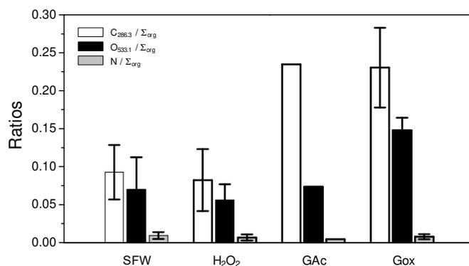
**Fig. 6.** Evolution of the molar concentrations ratioed to the sum of organic elements ( $\Sigma_{\text{org}} = \text{C} + \text{O}_{\text{org}} + \text{N}$ ) measured by XPS (data from Table 3) on 90Cu-10Ni samples after immersion
