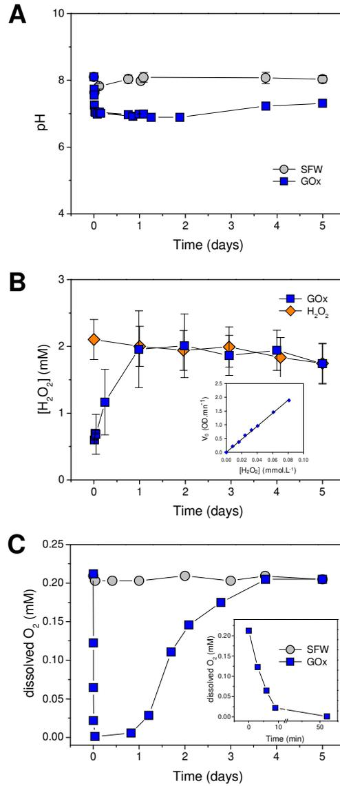
**Fig. 1.** Evolution of (A) pH, (B) concentration of H<sub>2</sub>O<sub>2</sub>, [H<sub>2</sub>O<sub>2</sub>], and (C) dissolved O<sub>2</sub> as function of time during 5 days in (●) SFW, (◆) H<sub>2</sub>O<sub>2</sub> and (■) GOx media, as indicated. (B, inset) relationship between the activity of peroxidase (initial velocity V<sub>0</sub>) and the concentration of H<sub>2</sub>O<sub>2</sub>.
