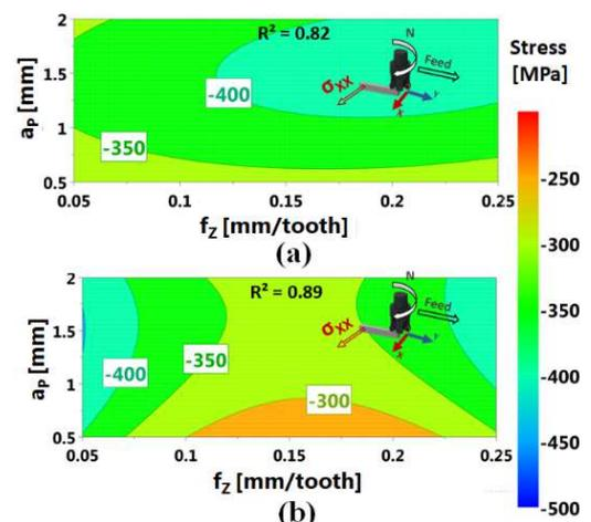
Fig. 8. Residual stress of (a) the conventional and (b) LMD parts measured in the cutting direction  $\sigma_{xx}$  (contour plot).
