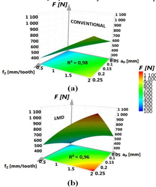
finer grains that are found in the AM parts. The higher cutting forces are a result of a greater load on the cutting tool which could lead to a low machinability of the material and higher tool wear.
