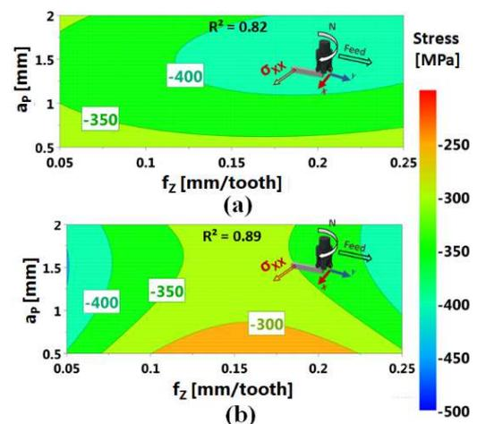
Fig. 8. Residual stress of (a) the conventional and (b) LMD parts measured in the cutting direction  $\sigma_{xx}$  (contour plot).
