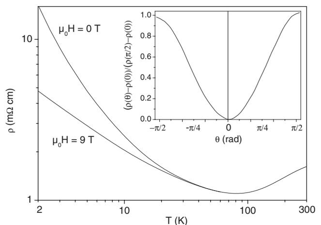
FIG. 1. Temperature dependences of the single crystal in-plane resistivity  $\rho$  at 0 T and 9 T, the magnetic field being parallel to the  $\text{CoO}_2$  planes. The inset displays the variation of the normalized magnetoresistance with the angle between the  $\text{CoO}_2$  planes and the 9 T magnetic field at  $T=60$  K.
