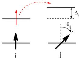
FIG. 5. (Color online) Schematic picture of the electronic energy levels involved in an elementary spin dependent hopping from site  $i$  to site  $j$ . The magnetic potential barrier  $\Delta_{ij}$  results from the misorientation  $\theta_{ij}$  between the quasiparticle spin  $s_i$  (thin red arrow) and the localized spin  $\sigma_j$  (bold black arrow) as explained in the text.
