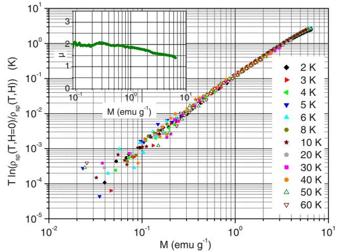
FIG. 6. (Color online) Scaling plot of the effective single crystal in-plane magnetoresistance  $\rho_{sp}(T,H)$  as a function of the magnetization over the whole temperature range. Here,  $\rho_{sp}(T,H)$  has been calculated by subtracting from the experimental value a constant resistivity at each temperature above 10 K. To make sense, the subtracted part is assumed to be weakly magnetic field dependent. The inset displays the variation of the exponent  $\mu$  with the magnetization.
