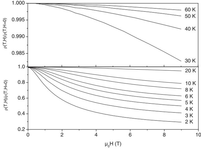
FIG. 2. The upper and lower panels display the magnetic field dependences of the normalized resistivity  $\rho(T,H)$  over the whole investigated temperature range, the magnetic field being parallel to the  $\text{CoO}_2$  planes.
