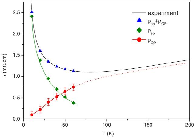
FIG. 7. (Color online). Temperature dependences of the experimental resistivity, the subtracted metalliclike part  $\rho_{QP}$  and the deduced insulatinglike part  $\rho_{sp}$ . The dotted line is an extrapolation to recover the high-temperature metalliclike behavior.
