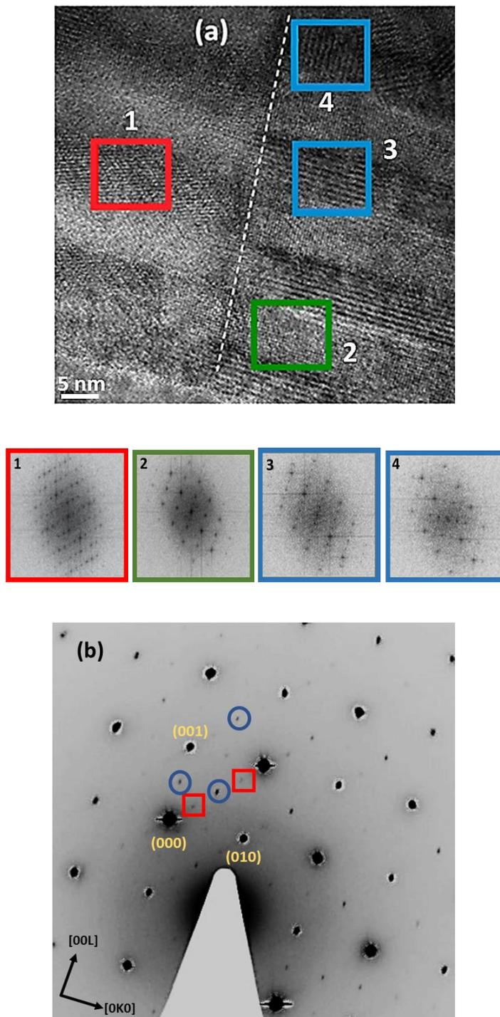
Figure 4: (a) High resolution TEM image for SL with  $\Lambda = 150 \text{ \AA}$  ( $N=5$ ). The red square indicates the  $45^\circ$  dense lamellar only present in the BFO layers (periodicity of 1.15 nm), the green square shows any regions which reveal no domain structure in the BFO layers suggesting a pseudo-cubic unit cell. The blue squares highlight the horizontal and vertical
