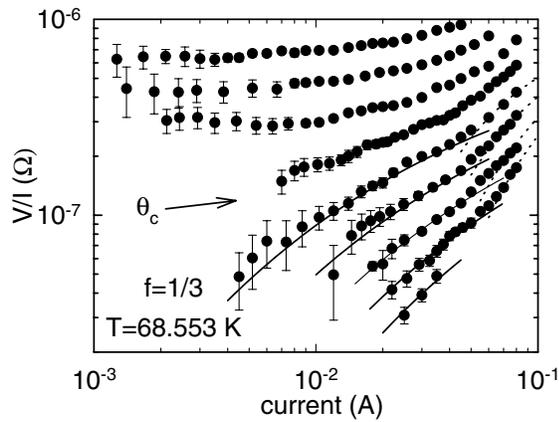
FIG. 1.  $V/I$ - $I$  curves for tilted magnetic fields. From the right to the left  $\theta = 0^\circ, 5^\circ, 10^\circ, 15^\circ, 20^\circ, 25^\circ, 30^\circ, 35^\circ,$  and  $40^\circ$ . The curved lines are a fit of the Bose glass theory to the data.
