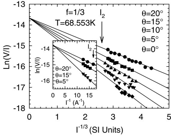
FIG. 3.  $\ln(V/I)$  vs  $I^{-1/3}$  for  $I < I_2$  and  $\theta < \theta_c$ . Inset:  $\ln(V/I)$  vs  $I^{-1}$  for  $I > I_2$  and  $\theta < \theta_c$ . In both plots the lines are a fit to the data using the form  $\ln(V/I) = P - Q_\mu I^{-\mu}$  with  $\mu = 1/3$  or  $1$  according to whether  $I$  is  $< I_2$  or  $> I_2$ .
