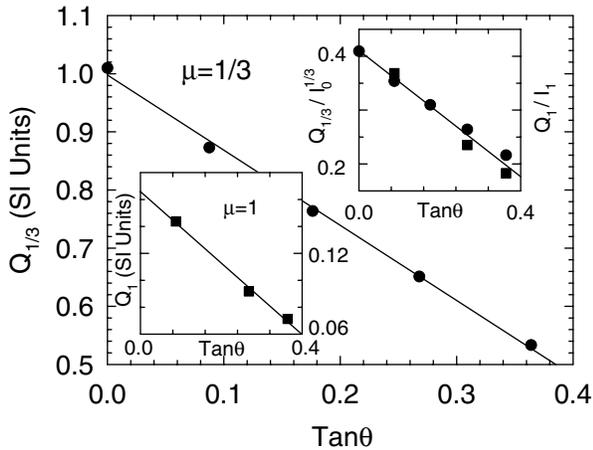
FIG. 4. Angular dependence of  $Q_{1/3}$  defined in the regime  $I < I_2$  (see Fig. 3). Lower inset: angular dependence of  $Q_1$  defined in the regime  $I > I_2$ . Upper inset: angular dependence of  $Q_{1/3}/I_0^{1/3}$  and  $Q_1/I_1$ . In each plot the straight line is a least-squares fit.
