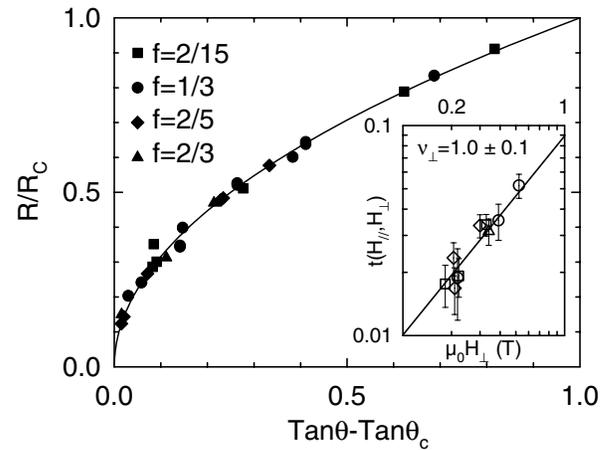
FIG. 5. Critical behavior of the linear resistance for different values of  $f$  and  $T$ . The curved line is a fit to the data using  $R = R_c(\tan \theta - \tan \theta_c)^{1/2}$  in accordance with a CIC transition scenario. Inset: angular dependence of the Bose glass transition. The solid line is a fit to  $T_{BG}(H_{\parallel}, 0) - T_{BG}(H_{\parallel}, H_{\perp}) \sim |H_{\perp}|^{1/\nu_{\perp}}$  with  $\nu_{\perp} = 1.0 \pm 0.1$  to the data; the point (0, 0) is included.
